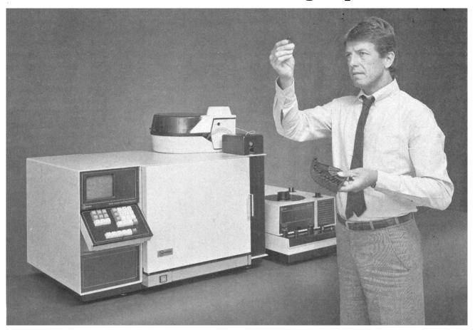
Varian Series 5000 HPLC instruments together with newly developed special high performance columns provide the protein chemist/biochemist/biologist with three chromatographic modes for the rapid separation of proteins and peptides:
